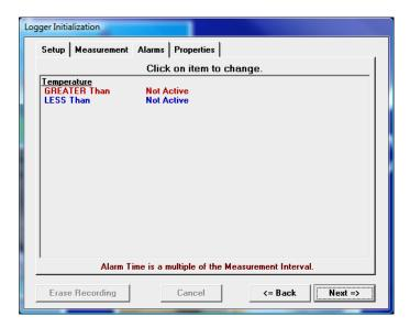
Check the High Alarm Limit or Low Alarm Limit if you want to enable the flashing LED alarm indicator.
