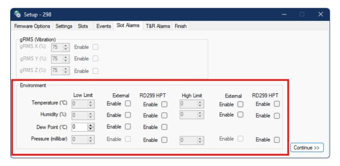
The user must continue to the "T&R Alarms" tab to configure tilt and roll alarms. This option is possible if the ShockLog 298 used has the capable hardware and the Tilt & Roll option is enabled on the "Firmware Options" tab.
